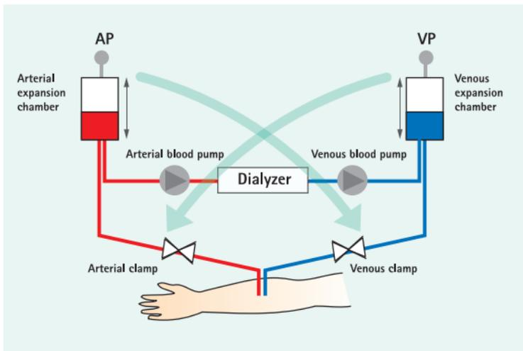
The Single-Needle Cross-Over (SN-CO) name is derived from the control's special feature: When reaching a certain control pressure, the opposite tube clamp closes and the respective other phase begins. Hence, the clamps' control is carried out crosswise: Cross-Over.
